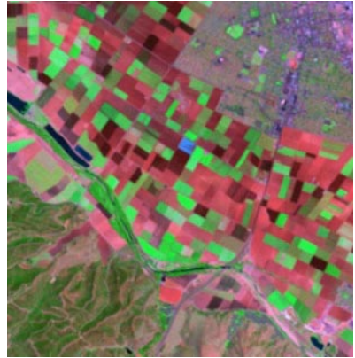
Color composite Landsat Thematic Mapper image with Red = TM7, Green = TM4, and Blue = TM2. Scene shows farmland flanked by an urban area (upper right) and grassy hills (lower left).
