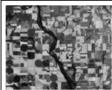
The cool river surface, its flanking wooded strips, and agricultural fields with full crop cover appear dark in this summer mid-morning thermal image of an area in Kansas (USA). Brighter fields are bare soil. From Landsat 7 ETM+, band 6, with 60-meter ground resolution.
